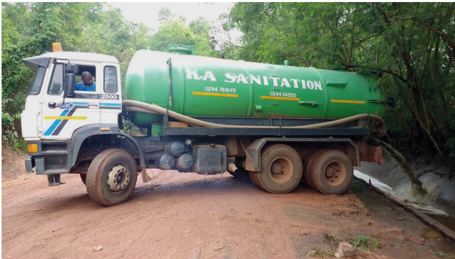
Vacuum tanker for emptying and transporting faecal sludge, Kumasi, Ghana.
