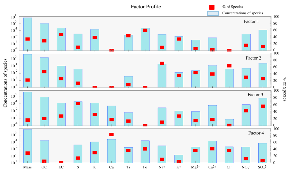
Figure 9. Source apportionments by positive matrix factorization (PMF) receptor model. (a) Source profiles for total suspended particles from PMF, (b) factor contributions from PMF in relation to sampling time, and (c) factor loading for TSP mass (yellow arrow: episode type I; gray arrow: episode type II).
