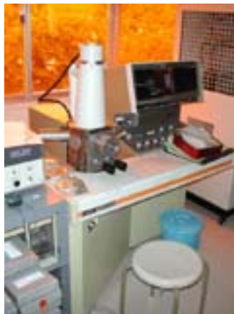
Figure 4.15: The picture of the scanning electron microscopy (SEM) machine - used in this research.
