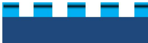
Figure 6.12: Schematic of the first approach - process of 2-D PhC structures before Si-ion implantation.
