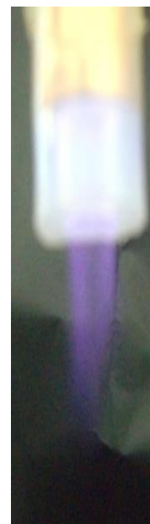
Figure 2.7 A stabilized homogeneous plasma discharge obtained by applying a sinusoidal voltage ( V_{pp} 20 kV) at the frequency of 20 kHz to the mixture of Ar (10 slm) and N 2 (100 sccm). The length of the jet was about 2.5cm.
