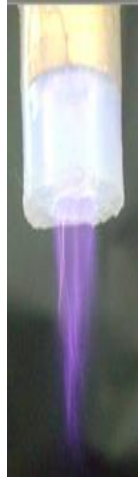
Figure 2.6 A highly filamentous discharge obtained by applying a sinusoidal voltage ( V_{pp} 20 kV) at the frequency of 20 kHz to Ar (10slm) only. The length of the jet was about 3.0cm.
