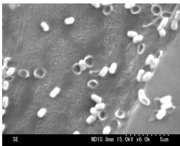
Figure 4.12 Bacillus subtilis spores after exposing to the homogeneous plasma discharge for 5 minutes.
