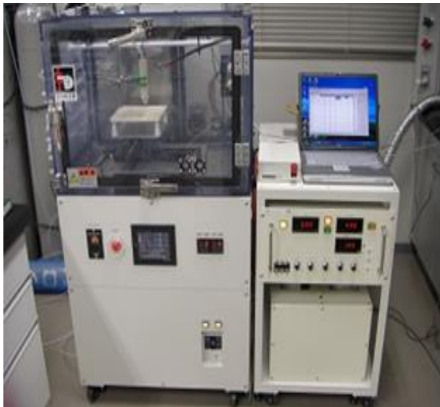
Figure 3.1 CAPPLAT (Cold Atmospheric Pressure Plasma Torch). This is the basic unit.
