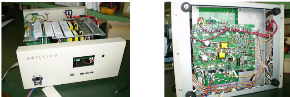
Fig.5. 1. Actual inverter power supply device
