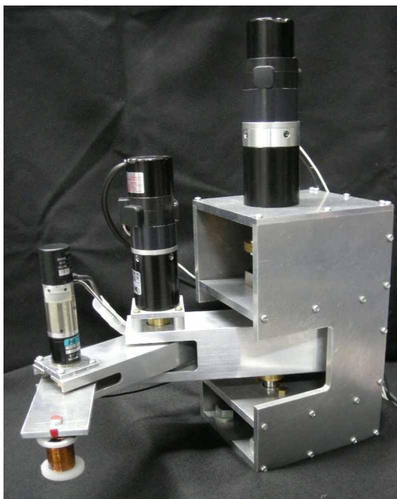
Fig. 2.1 Photograph of the three-link robot arm with Electromagnetic attraction hand
