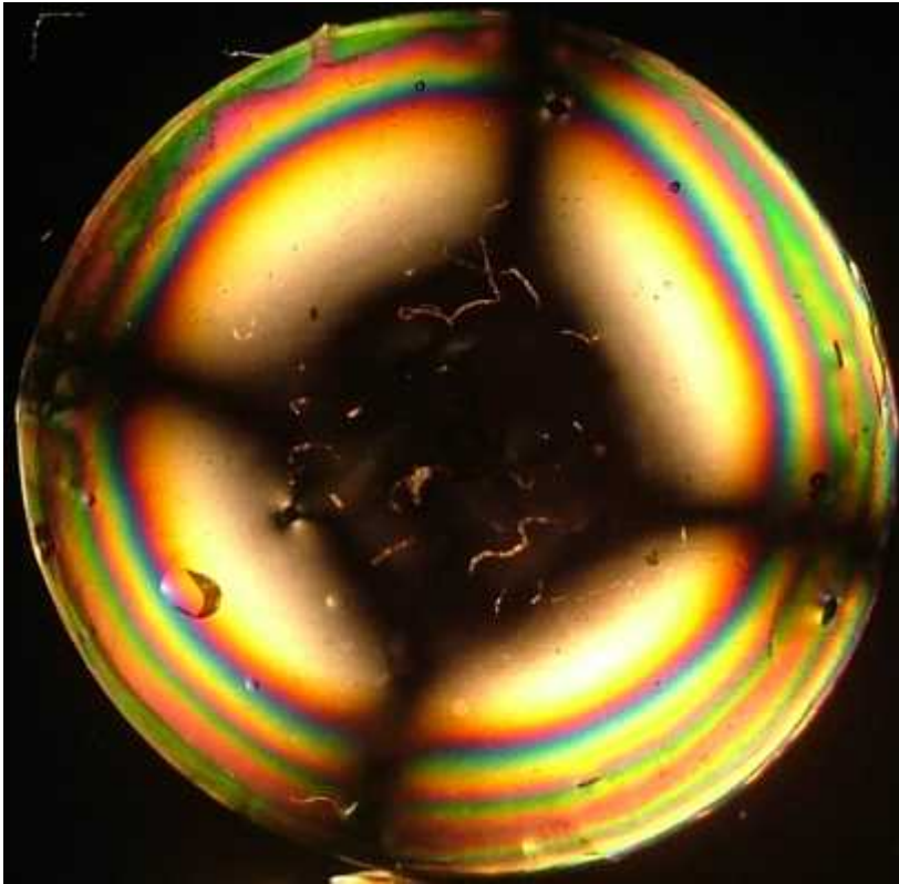
Figure 1. DNA liquid-crystalline gel observed from the upper view of the cross-sectional strip perpendicular to the long axis of dialysis tube under crossed nicols.
