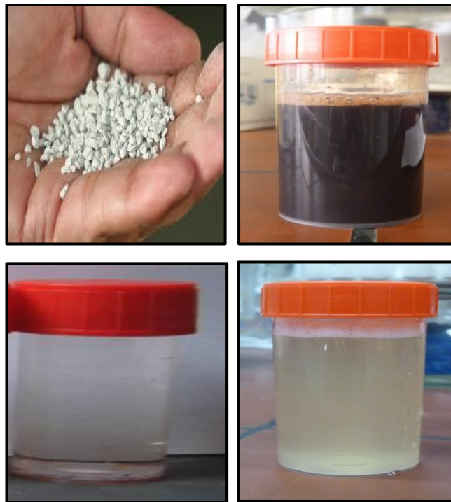
Struvite (top left), liquid fraction of digestate (top right), effluent from constructed wetlands (bottom left) and air scrubber water (bottom right) (Pictures: Sigurnjak, I.)
