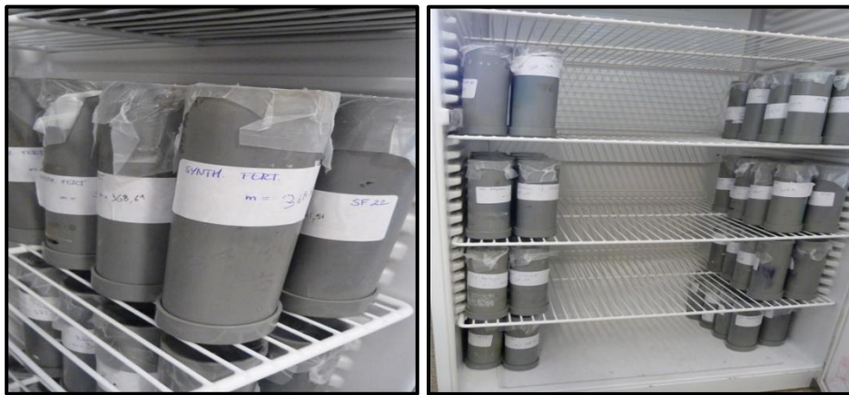
PVC tubes, containing mixture of soil and bio-based materials, incubated in 120-day incubation experiment (Pictures: Sigurnjak I.)
