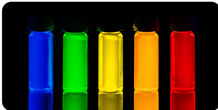
Figure 1.3: Photoluminescence of cadmium selenide (CdSe) QDs with particle diameters increasing from left to right.
