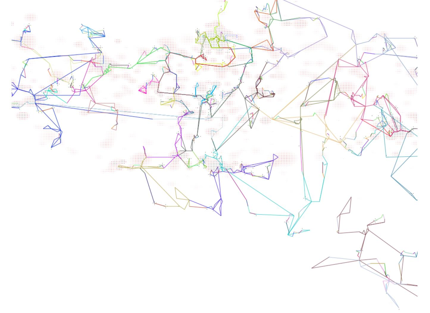
Generator phases: Position stops Connect stops with edges Create synthetic routes Instantiate timely trips Serialize to GTFS or RDF
