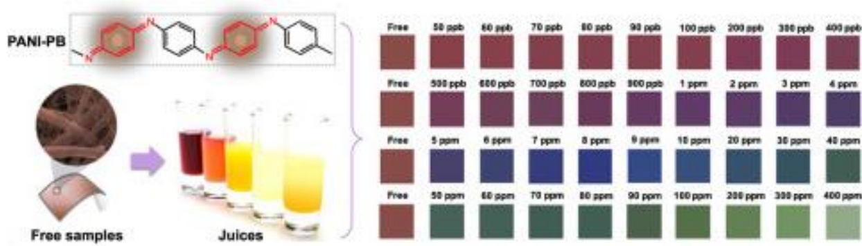
Figure 7. PA 66 is blended with PANI-PB for the production of colorimetric nanofibers that detect L-ascorbic acid in juices. A color differentiation map was constructed to link color to analyte concentration. Reproduced with permission. [156] 2015, Elsevier.
