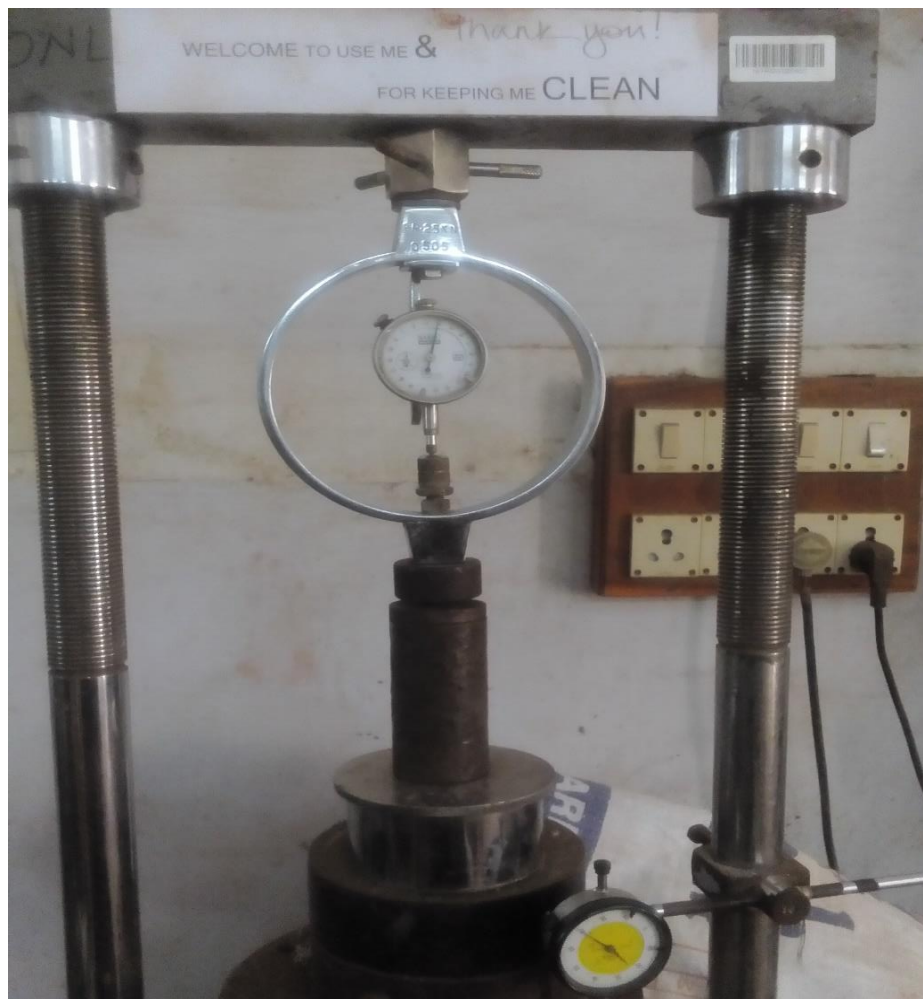
Fig 4.1 Experimental setup for UCS
