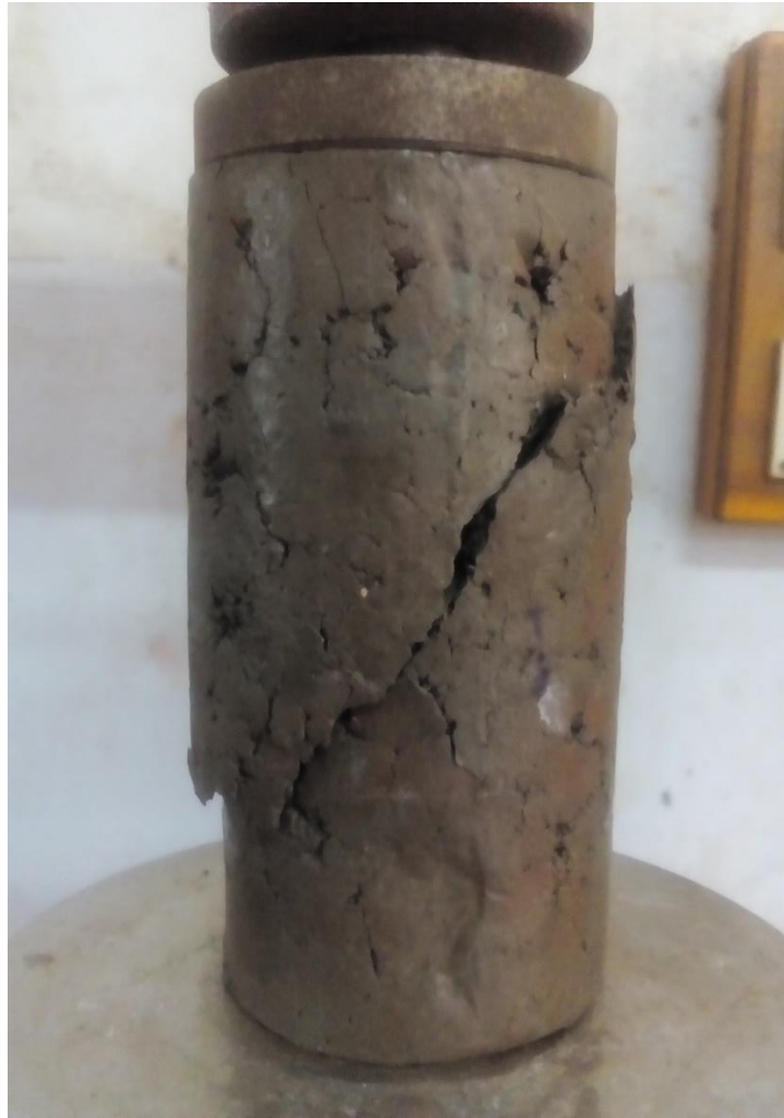
Fig 4.2 Failure pattern of the specimen
