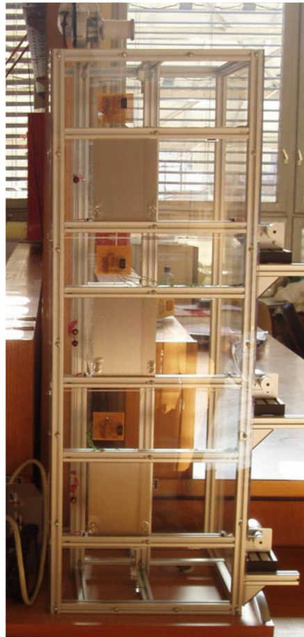
Figure 1: Profile construction of the personal lift.
