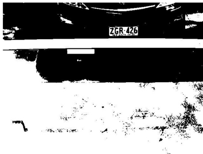
Figure 5: Image thresholded using global thresholding method
