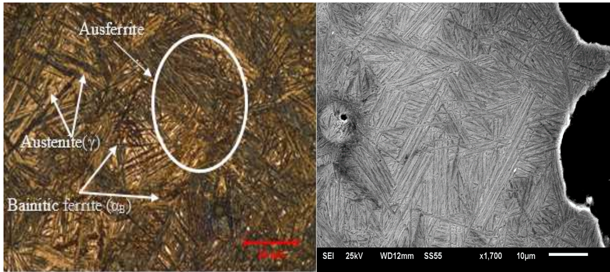
Figure.19(a): Optical and SEM micrograph of cryogenically treated ADI, T_{\gamma}=1700^{\circ}\text{F} , T_A=500^{\circ}\text{F}
