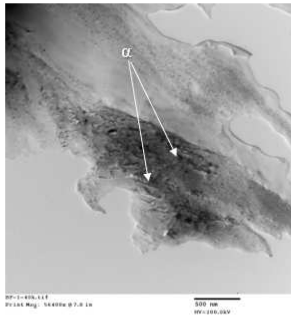
Figure.43: TEM micrographs showing Bright field image of plastically deformed ADI ( T_{\gamma}=1700^{\circ}\text{F} , T_D=1700^{\circ}\text{F} , T_A=725^{\circ}\text{F} )
