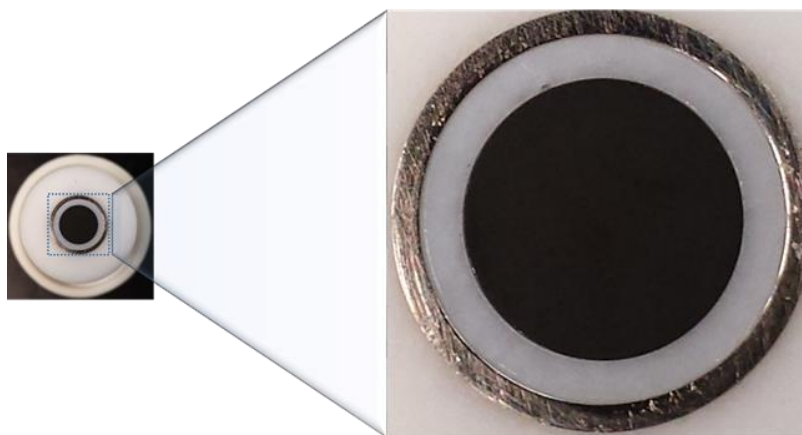
Figure 3.3 Catalyst/carbon thin-film deposited on glassy carbon disk electrode.
