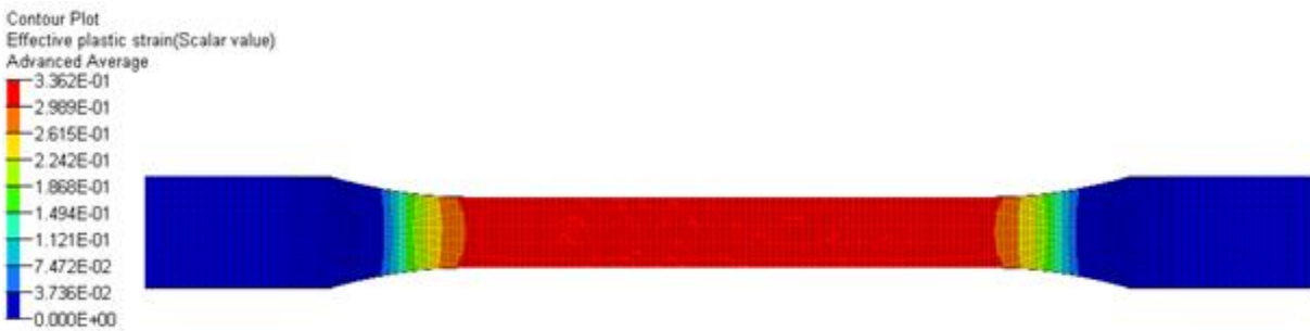
Fig 5.8. Strain (XX) Contour of Uniaxial Tension Specimen at Elongation Speed of 10 (mm/s)
