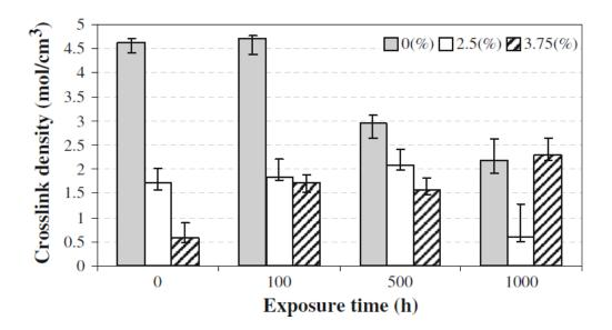
Figure 2.1.3 Crosslink density change after weathering with different loads of nano-silica (Yari et al., 2008).
