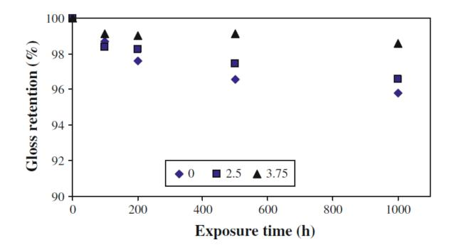
Figure 2.1.1 Gloss retention of clear coat containing different loads of nano-silica after various wreathing times (Yari et al., 2014).
