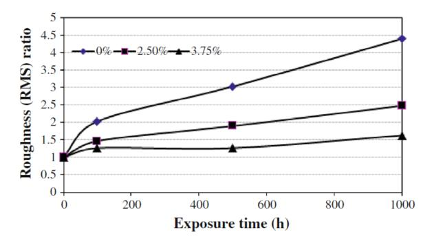
Figure 2.1.2 Roughness variation of different acrylic melamine clearcoat containing different loads of nano-silica during weathering (Yari et al., 2009).
