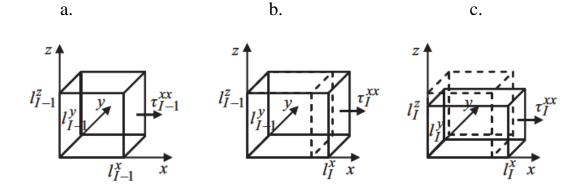
Figure 4.5.1 Sketch of a simulation box: (a) before imposing the *i*-th strain increment, (b) after imposing the *i*-th strain increment, (c) after the system relaxation (Xiao et al., 2009).
