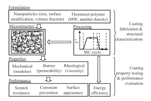
Figure 3.1 Multi-Scale Correlation establishment for Thermoset Nanocomposites (Xiao et al.,
