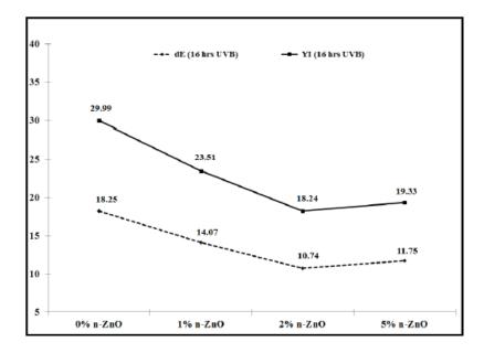
Figure 2.2.1 Color change and yellowness index after 16 hrs exposure respect to different percentages of flake-like ZnO load (Rajagopalan and Khanna, 2013).
