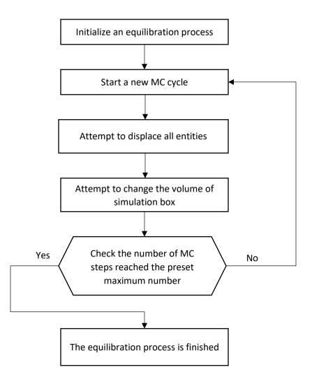
Figure 4.2 System equilibration flowchart.
