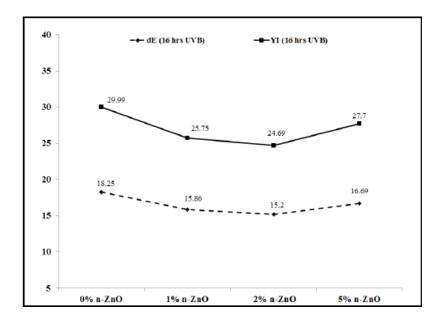
Figure 2.2.2 Color change and yellowness index after 16 hrs exposure respects to the different proportion of spherical ZnO amount (Rajagopalan and Khanna, 2013).
