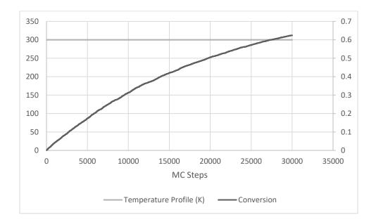
Figure 5.3.4 Nano coating curing process only under room temperature.
