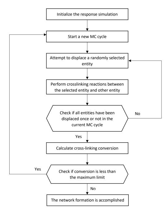
Figure 4.3 Cross-linking reaction flowchart.
