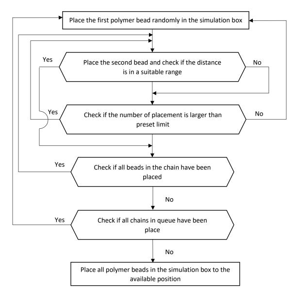
Figure 4.1 System initializing flowchart.
