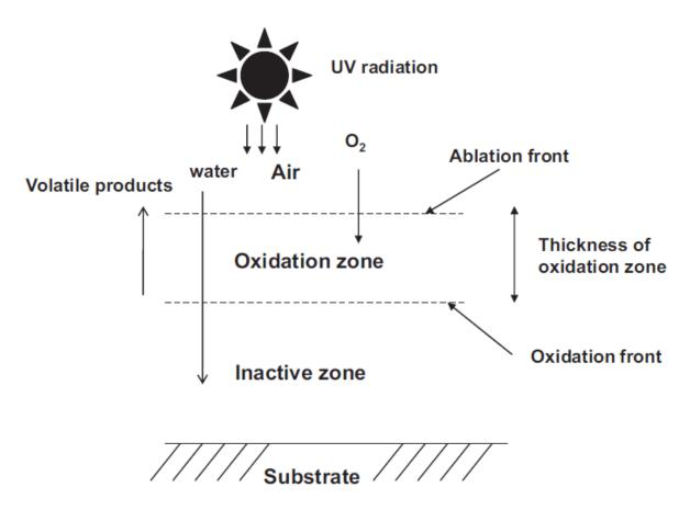
Figure 3.2 Schematic illustrations (cross-section view) of the epoxy-amine coating during exposure to ultraviolet radiation and humidity (Kiil, 2009).
