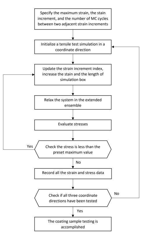
Figure 4.5 Coating testing simulation process flowchart.
