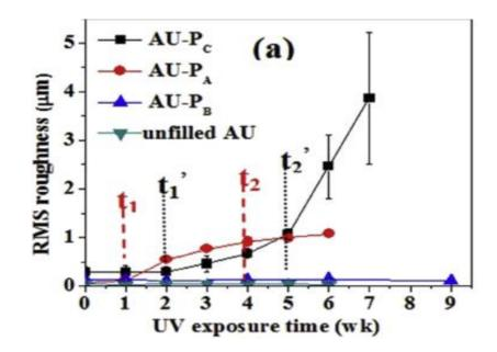
Figure 2.3.1 RMS roughness change respect to exposure time with different TiO<sub>2</sub> crystal type
