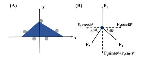
Figure 18 (A) The relative position of the glass and the columns. (B) The force analysis of the glass under the pressure of columns on the centering table.
