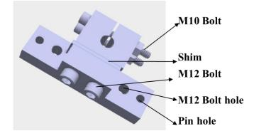
Figure 22 The structure of the new design of the column base.
