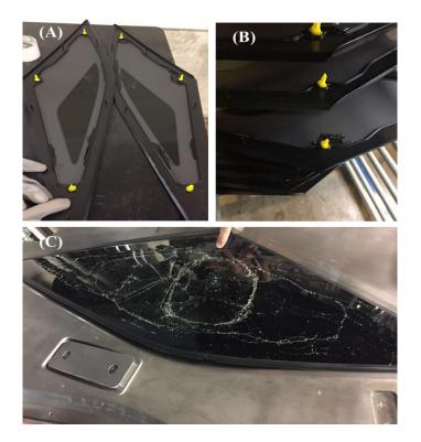
Figure 10 Low quality of the glass fabricated by the current centering table. (A) injection flash because of dislocation in the centering table, (B) large deviation, (C) chunk glass in the mold because of dislocation in the centering table.
