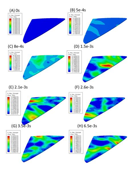
Figure 13 The maximum stress distribution of the glass at different times.
