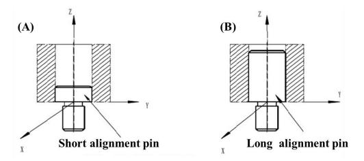
Figure 21 the schematic of (A) a short alignment pin and (B) a long alignment pin.
