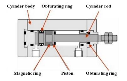
Figure 19 The structure and components of the traditional air cylinder.
