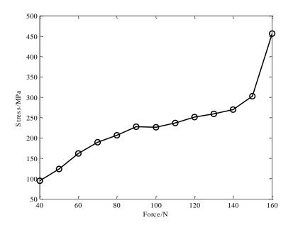
Figure 16 The stress variation of the glass under different impetus from the air cylinders.
