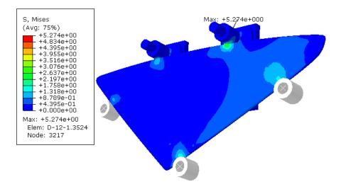
Figure 17 The stress distribution on the glass on static state with an impetus of 80N.
