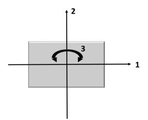
Figure 5 A rigid body in an x-y plane with 3 degrees of freedom.
