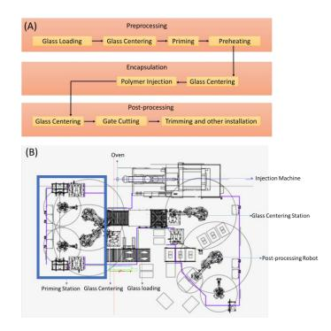
Figure 3 (A) Schematic of the traditional glass automation assembly procedure. (B) Schematic of a typical automatic assembly line.
