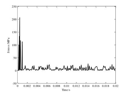
Figure 14 The variation of stress on the glass vs. time.
