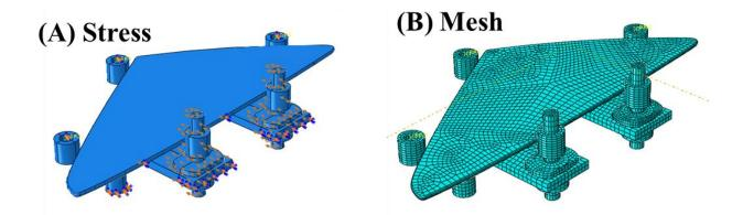
Figure 12 (A) The stress condition and (B) of the system based on finite element analysis.
