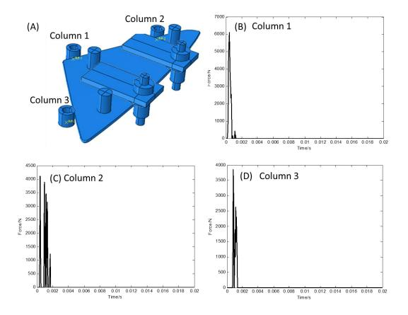
Figure 15 (A) The bottom view of the centering system shows the locations of the three fixed columns. (B), (C), and (D) illustrate the variation of force on column 1, column 2, and column 3, respectively.
