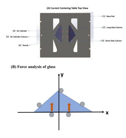
Figure 8(A) a schematic of the structure of the current centering table and (B) A schematic of the force analysis of glass on the centering table.
