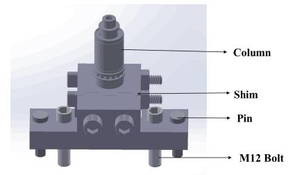
Figure 23 The schematic of the column base after assembling the column.
