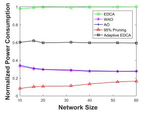
Figure 5.18: Comparison of Power Consumption with 95% Pruning vs. Other Solutions
