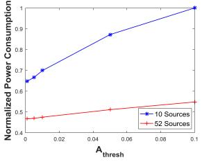
Figure 5.3: Power Consumption at Various Athresh Values
