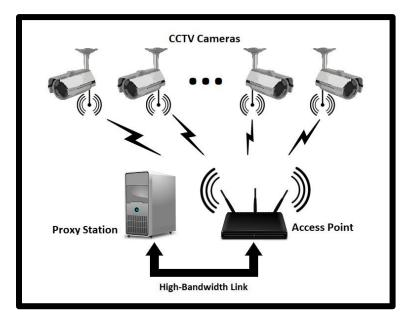
Figure 1.1: An Illustration of an Automated Video Surveillance System
