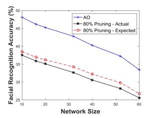
Figure 5.12: Expected vs. Actual Facial Recognition Accuracy at 80% Pruning
