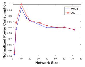
Figure 5.8: WAO vs. AO Comparison of Power Consumption
