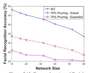
Figure 5.13: Expected vs. Actual Facial Recognition Accuracy at 70% Pruning
