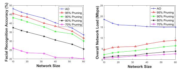
Figure 5.9: Comparison of Facial Recognition Accuracy at Various Pruning Levels
