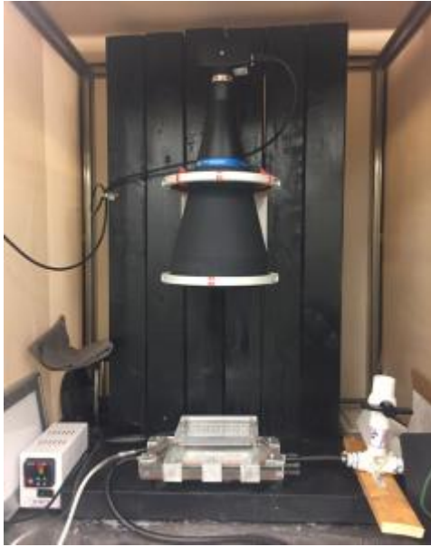
Figure4: The camera, lens and the 24-well plate setup for the swimming behavior of daphnia pulex and danio rerio .
