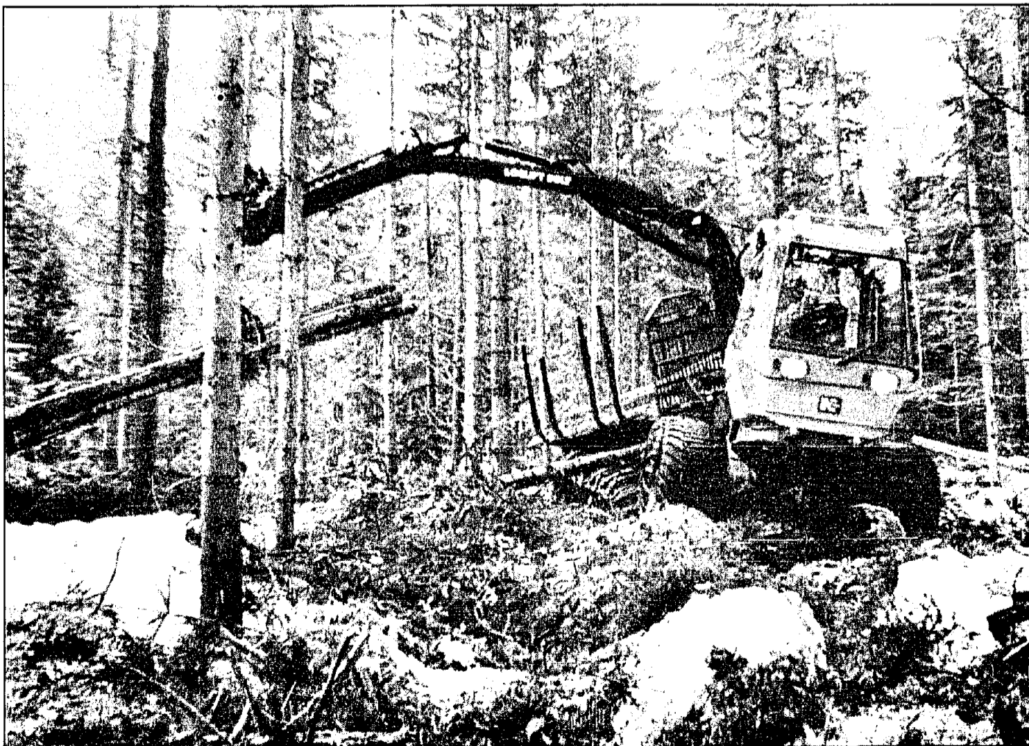
THE THINNINGS felled, delimited and cut to length, this self-loading machine moves in to pick up the wood and take it out to
