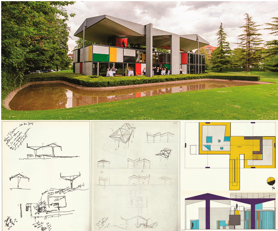
Figure 4. Pavilion Heidi Weber, Center Le Corbusier, Zurich. First sketches, studies on the geometries of the two covers and supporting pillars. The relationship between the roof structure and the architectural spaces - plant and section.
