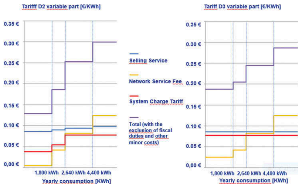
Figure 4. Electricity tariff breakdown (variable part) before the reform for a resident and non-resident customer (Energy&Strategy 2016a).
