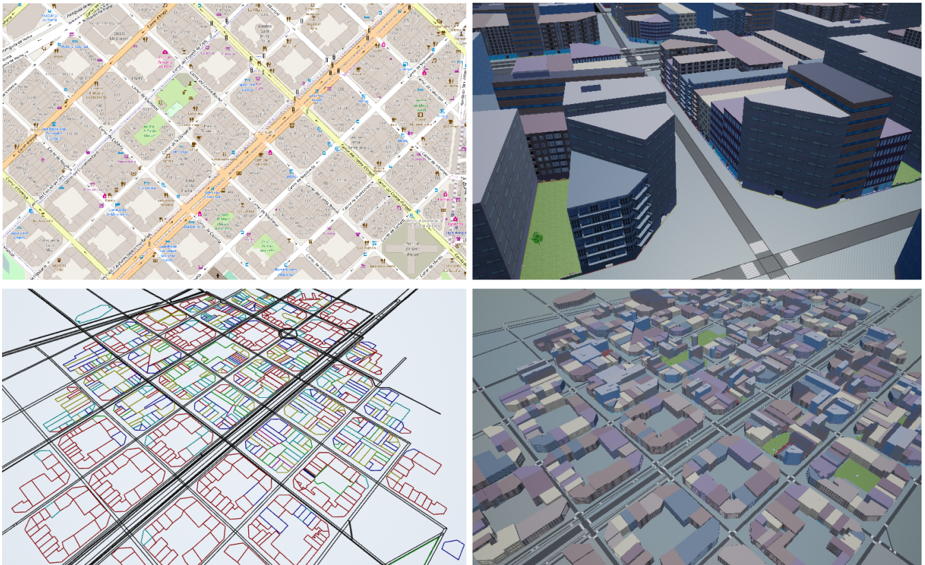
Figure 4: Generation of a section of the city of Barcelona. Top Left: input OSM data as seen in the official web page. Bottom Left: the generated layout (lots and road network), where each color represents a different lot type (usage). Bottom Right: aerial view of result after the CGA generation. Top Right: a close-up of the result.
