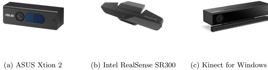
Figure 3.4: Consumer range imaging devices. Sources: [5], [15], [11]
