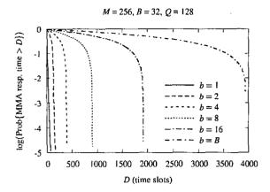
Fig. 4. Complementary distribution function of the MMA response time for Q = 128 and different values of b.
