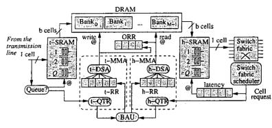
Legend: RR: Requests Register ORR: Ongoing Requests Register BAU: Bank Allocation Unit QTR: Queue Transfer Requester DSA: DRAM Scheduler Algorithm MMA: Memory Management Algorithm
