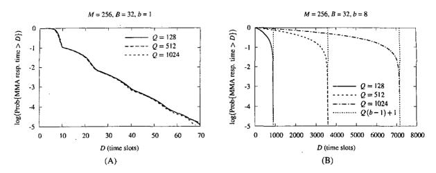
Fig. 3. Complementary distribution function of the MMA response time for different values of Q and b = 1 (A), and b = 8 (B).
