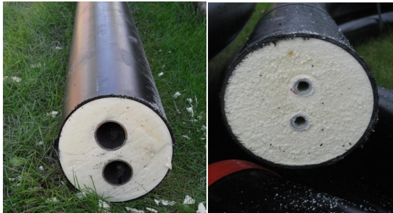
Figure 3-4 Example of district heating twin pipes. A steel pipe twin pipe (DN50) 60-60/225 mm (left) and a flexible pipe 14-14/110 mm 140
