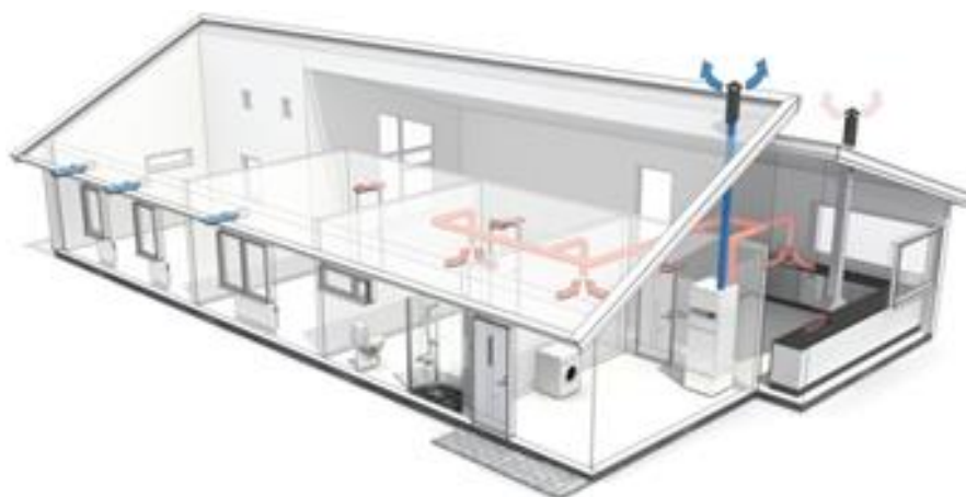
Figure 2-10: Electrical heat pump, ventilation 76
