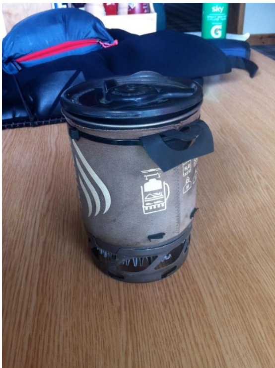
Appendix 3.6: Image of modified jet boil (for expedition cooking)
