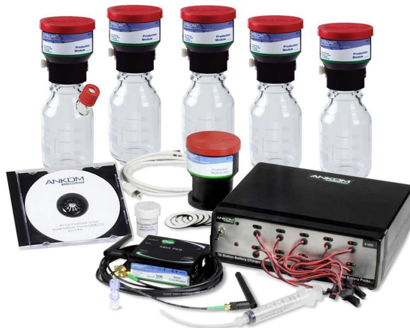
Figure 2.6 ANKOM RF Gas measurement system, used for measurement of cumulative carbon dioxide gas measurement.
