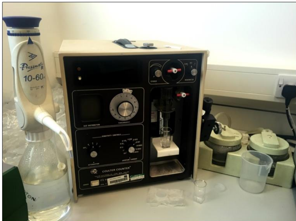
Figure 2.4 Coulter Counter used to enumerate yeast cell number/ml
