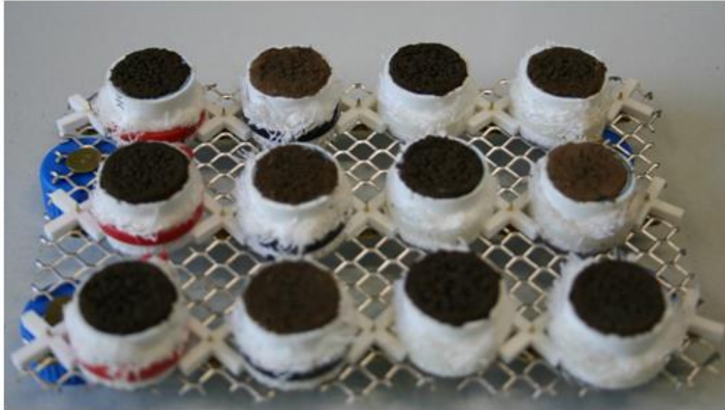
Figure 6.2: Arrangements of soil samples for resin impregnation. The soil rings were tied with different color bands in order to easily distinguish between treatment samples after impregnation, here shown for an experiment where red color stands for soil packed at 1.3 \text{ g cm}^{-3} , black stands for soil packed at 1.5 \text{ g cm}^{-3} and white color stands for control samples.
