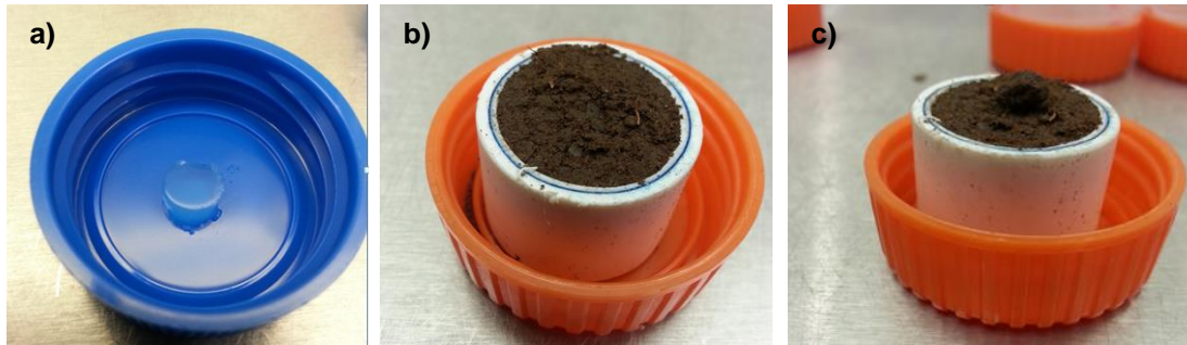
Figure 4.1: Experiment setup to quantify bacterial spread in soil. An agarose bead prepared with bacterial inoculum and agarose solution was used as a source. It was placed at the bottom of the soil sample. A single 2-4 mm aggregate was used as a bait to quantify successful colonisation of the soil. The bait was placed on the top of the sample.
