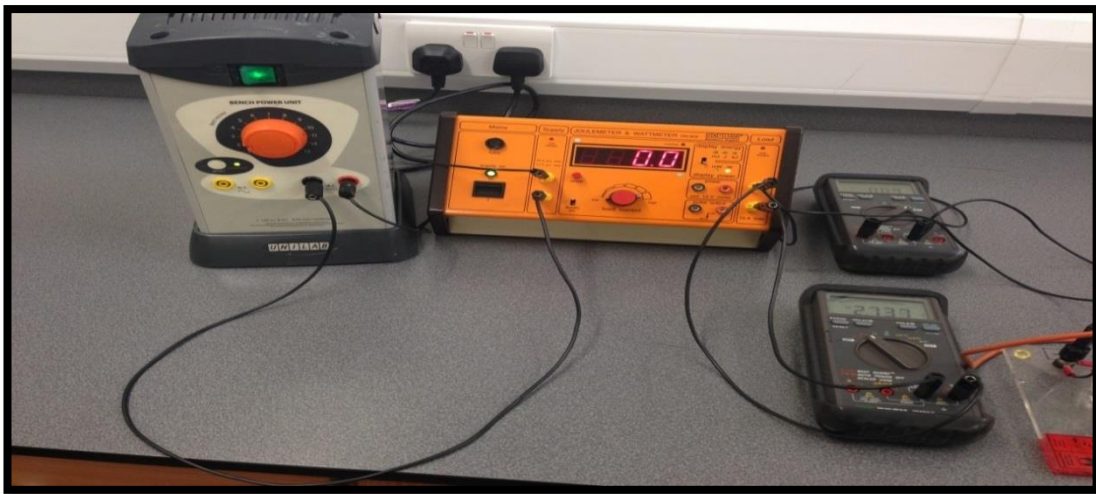
Figure 4.15: Digital Joule-meter and wattmeter with electrolyser connections.
