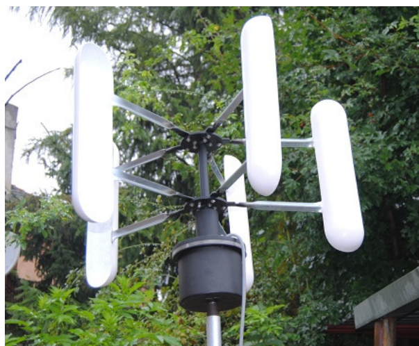
Figure 4. The prototype carousel-type vertical axis wind turbine C-VAWT designed for the powering of the developed APS system
