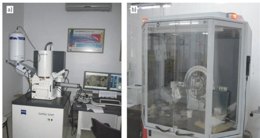
Figure 1. a) SEM-EDS test machine; b) XRD test machine
