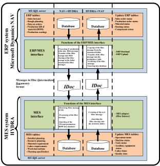
Figure 1 Conceptual model of MES and ERP systems integration
