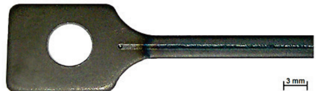
Figure 7 Testing specimen after welding
