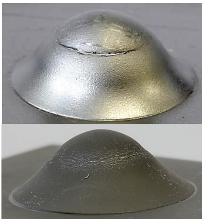
Figure 4 Erichsen cupping test: DC 01 (top) and PLASOX process (bottom)
