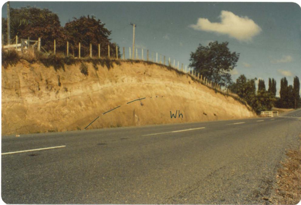
Fig. 2.27 Cover deposits overlying Whakamaru Ignimbrite on Whites Road. The Kawakawa Ash is shown by a distinct white layer in the middle of the cutting.
