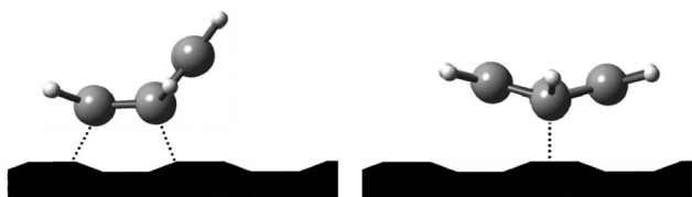
Fig. 8 Side views for tight bridge (left) and butterfly (right) configurations of benzene adsorbed on the Si(001) surface. Gray and white spheres are C and H atoms, respectively. Adapted from ref. 94.
