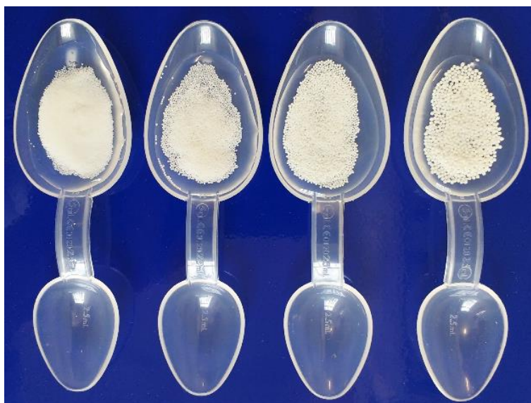
Figure 3.2. Samples of 500 mg of multiparticulates dispersed in 3 ml of spring water on a medicine dosing spoon. Particle size of the multiparticulates varies, from left to right: 200-355, 350-500, 500-710 and 700-1000 µm. Each size was available as coated and uncoated versions.
