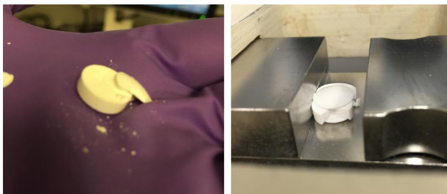
Figure 5.4. Capping post-tableting (left) and after hardness testing (right), observed for tablets prepared using Pearlitol Flash and SmartEx QD50 at high compression forces ( > 200 MPa).
