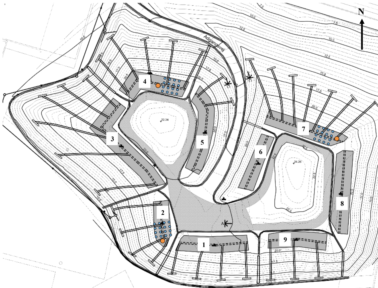
Figure 1. Cell 0 seen from above. The grey boxes indicate the biocover sections. Pipes can be seen on the slopes of the landfill, feeding landfill gas to the sections. Blue dots represent the approximate position of the measuring points, though the area they cover is exaggerated. Orange dots represent the approximate position of the excavation sites.
