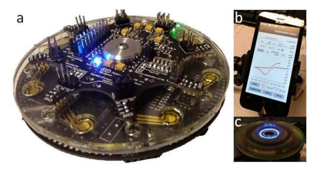
The first application of the PLoD is a potentiostat for electrochemical based biosensing [1], we have successfully measure Ferri Ferrocyanides Current-Potentio curve while spinning from 0 to 3000 rpm. There are various lab-on-disc applications[2] can be carry out by the PLoD platforem for the future stand-along diagnostics and healthcare systems.
