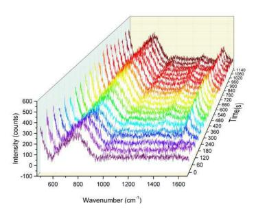
Figure 1.Operando Raman results showing graphite formation on Ni-STN based electrode at
