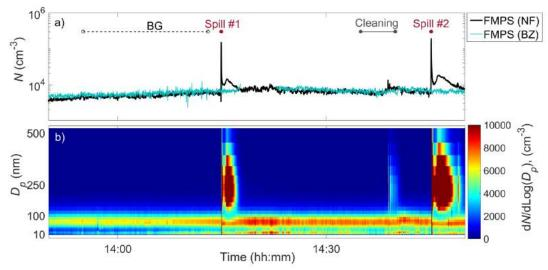
**Figure 1** (a) Particle number concentration measured at near field (NF), and breathing zone (BZ) during spillage of 60 g of ultrafine TiO<sub>2</sub>; (b) particle number size distribution measured in NF.
