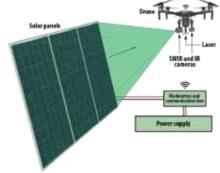
Fig. 1. Concept of automated drone inspection.
