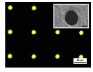
Figure 2. Microscope dark field image of a 2x2cm 2D holes grating made in 50  $\mu$ m thick tungsten substrate using laser ablation. Insert: SEM image of 17  $\pm$  0.5 $\mu$ m  $\emptyset$  holes. Scale 5 $\mu$ m.
