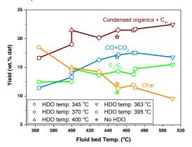
**Figure 2**: Effect of the fluid bed temperature.
