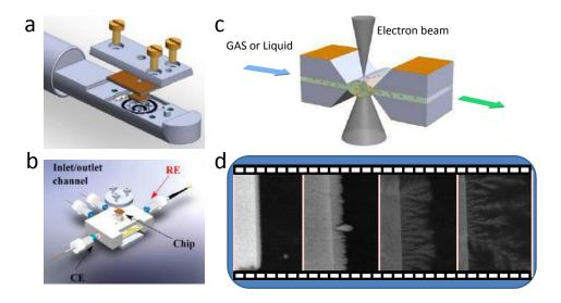
Figure 1, Schematic diagram of a SiNx membrane based chemical/electrochemical cell for catalysis process study, **a**: TEM cell; **b**: SEM cell; **c**: schematic illustration of window region and STEM imaging; **d**: in-situ electrodeposited copper with different morphologies (phosphate tuned) show high formic acid selectivity for CO2 reduction [1].
