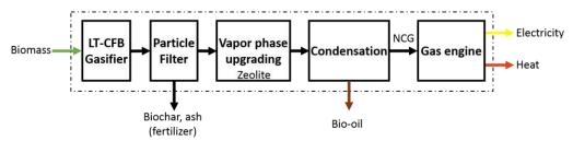
Figure 1: Process scheme of polygeneration plant comprised of various technologies.
