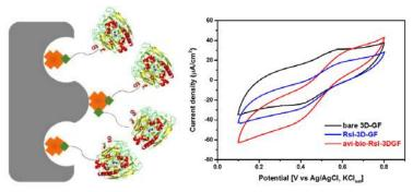
**Figure 1.** Schematic illustration of covalent immobilization of laccase on 3D graphene foam and its electrochemical behavior. Not drawn to scale.
