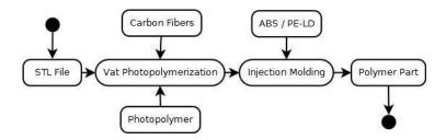
Figure 1 Overall process cycle with inputs and outputs.
