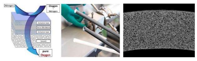
a) Schematic illustration of an oxygen transport membrane. b) Tubular oxygen transport membranes developed at DTU Energy. c) SEM cross section of a tubular oxygen transport membrane.
