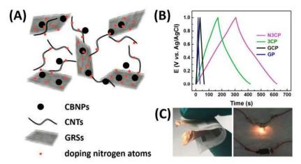
Fig.1 (A) Schematic for the heterostructure of the prepared nitrogen-doped multi-dimensional carbon materials. (B) Charge-discharge curves of different paper electrodes at 1 A·g<sup>-1</sup>. (C) A lab-made N3CP based flexible supercapacitor (left) and a miniature bulb is lightened up by such a flexible supercapacitor (right). Not drown to scale.
