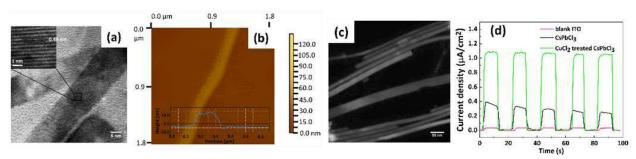
Figure 1. Characterizations of CuCl<sub>2</sub> pretreated CsPbCl<sub>3</sub> nanowires: (a) TEM image, (b) AFM image, (c) STEM image, and (d) comparison of photocurrent responses obtained at various photoelectrodes.
