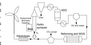
**Figure 1:** Simplified process diagram including fluid bed catalytic hydropyrolysis, char separation, temperature adjustment, vapor phase HDO reactor, cooling, condensation and liquid separationSteam reforming and water gas shift (WGS) of non-condensable gasses to produce H<sub>2</sub> and wind-powered electrolysis of water to H<sub>2</sub> is envisioned.
