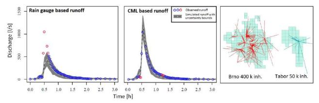
Fig. 1 – Left and middle: Runoff simulated based on three rain gauges about 2.5 km form the catchment located in Prague (CZ) in comparison to the runoff simulated from CMLs. Blue circles depict observed runoff inside of uncertainty bounds whereas red circles are outside of them. Right: CML topology in a city with 50 and 400 thousand inhabitants.
