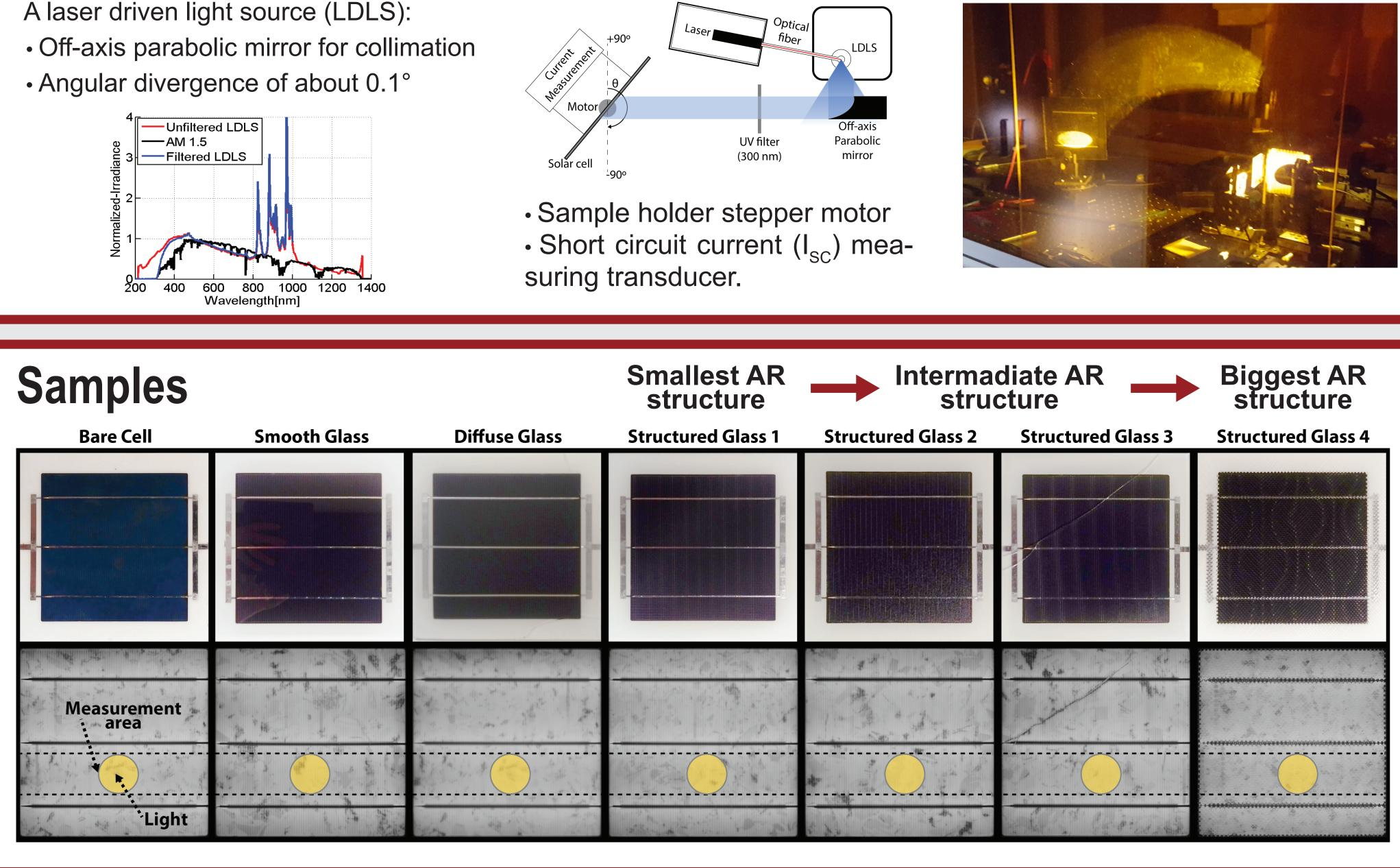
In this work, we normalize the relative short circuit current to a cosine response thereby isolating the optical effect of the glass-air interface. This form of data presentation is frequently described as the "incidence angle modifier" (IAM) and is used in PV modelling programs such as PVsyst.
