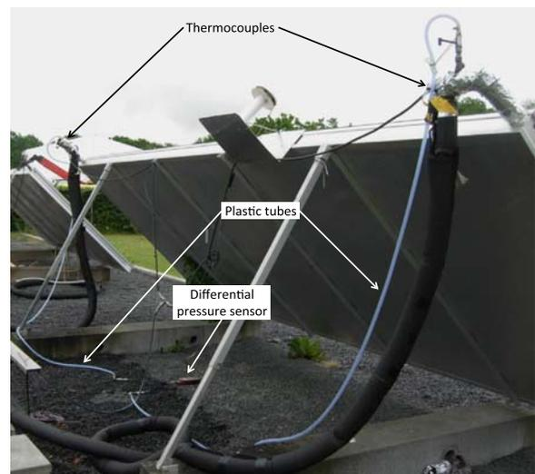
Fig. 2. Back of the HT-SA 35/10 solar collector with plastic pipes arrangement for pressure drop measurement.
