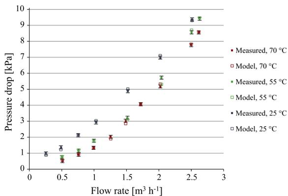
Fig. 5. Comparison between measured and calculated pressure drops for 50% propylene glycol/water mixture.
