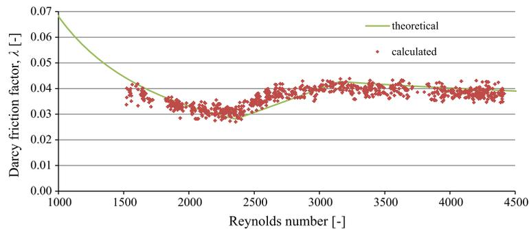
**Fig. A1.** Comparison between theoretical and calculated Darcy friction factor. The theoretical friction factor curve is obtained from (Eq. (7)) for  $Re < 2300$ , (Eq. (8)) for  $Re > 3100$  and linear interpolation between the two in between these values.
