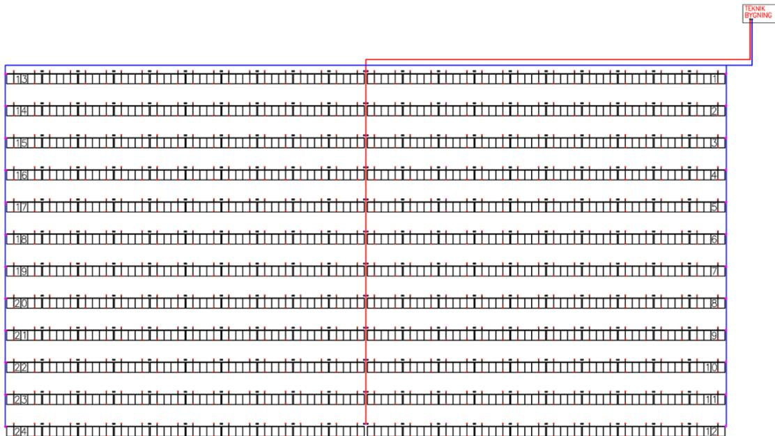
Figure 2: Layout of Høje Taastrup solar collector field: blue and red lines represent supply and return pipes respectively (adapted from Arcon-Sunmark A/S).
