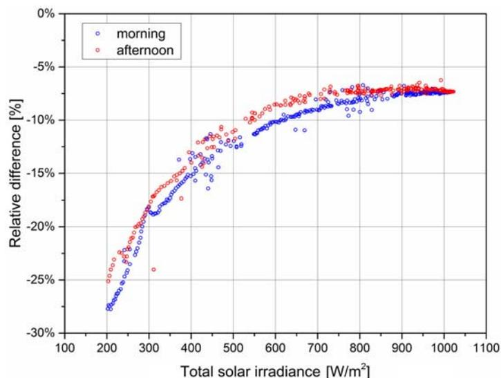
Figure 4.3: Relative difference in solar irradiance between silicon cell and thermopile pyranometer. The imperfect overlap of morning and afternoon data was likely due to slightly different orientations of the pyranometers.
