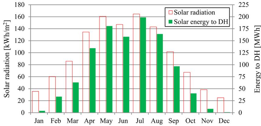
Figure 4: Monthly solar radiation on the collector plane (left axis) and solar energy delivered to the DH network (right axis) in the reference case.
