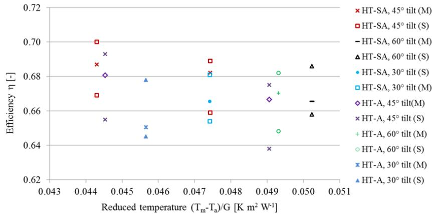
Fig. 7: Comparison between measured (M) and simulated (S) efficiencies of HT-A and HT-SA collector for a flow rate of 25 (litres min<sup>-1</sup>) and Reynolds numbers between 2200 and 2400. In each couple of simulated efficiency points the higher was obtained for turbulent flow and the lower was obtained forcing the Soleff models to assume laminar flow conditions.
