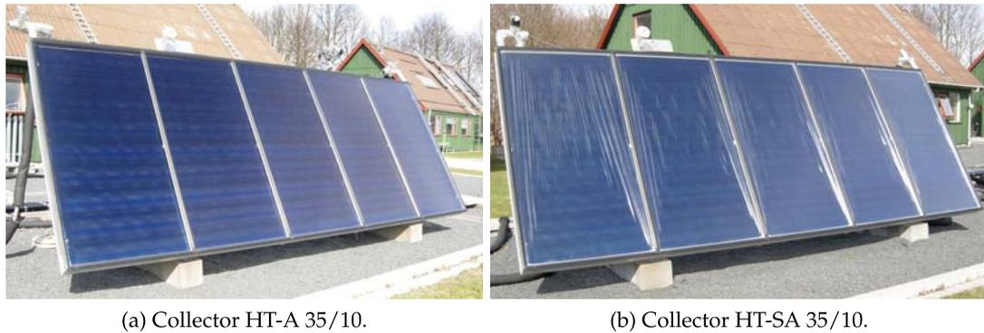
Figure 2.1: Tested solar collector HT-A 35/10 (a) and HT-SA 35/10 (b) at the Department of Civil Engineering at the Technical University of Denmark.
