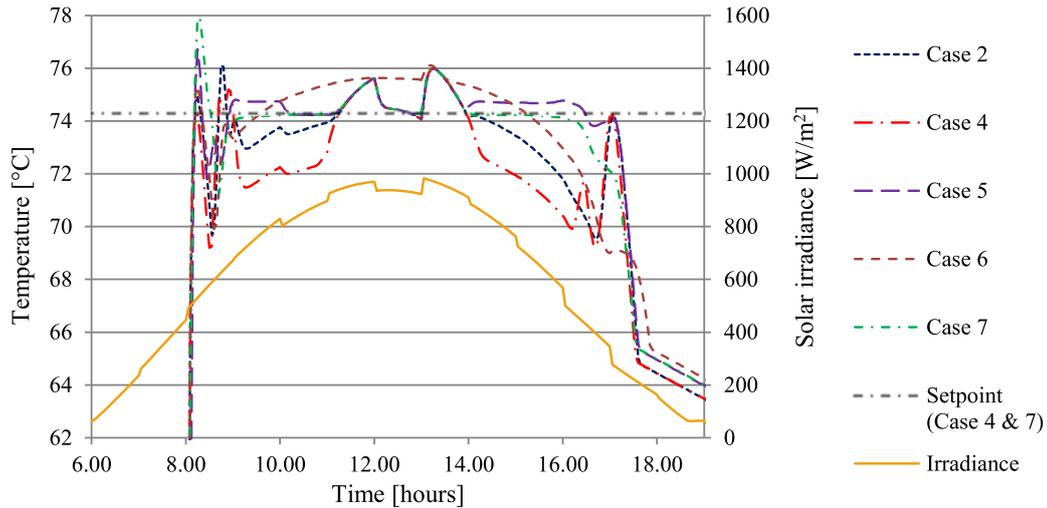
Figure 5: Outlet temperature from the collector field (Cases 2 and 4–7) and solar irradiance on the collector plane on June 7<sup>th</sup>.
