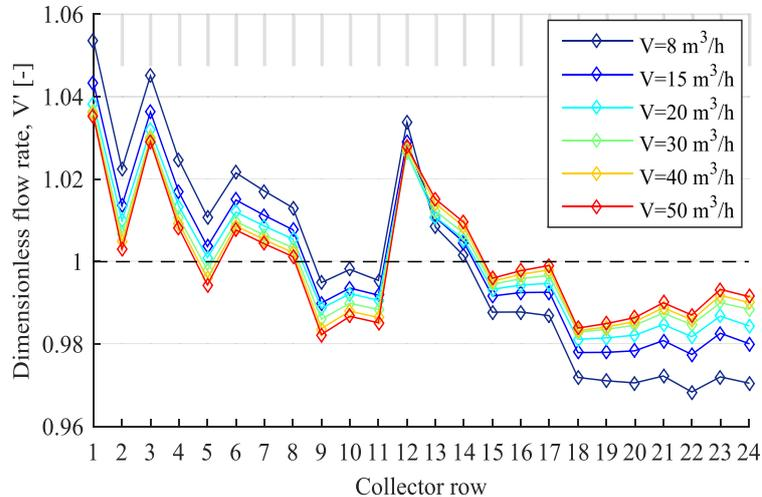
**Fig. 7: Modeled flow distributions in Høje Taastrup solar collector field for different field flow rates, assuming normal operating conditions (case 1).**
