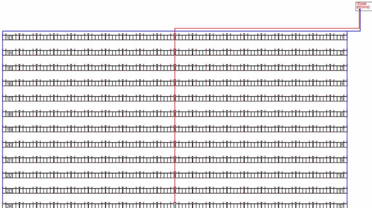
**Fig. 3.** Layout of Høje Taastrup solar collector field. Blue and red lines represent supply and return pipes respectively (adapted from Arcon-Sunmark A/S). (For interpretation of the references to colour in this figure legend, the reader is referred to the web version of this article.)
