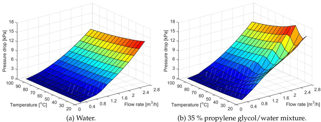
Figure 3.2: Pressure drop in Arcon-Sunmark HTHEATstore 35/08 collector.
