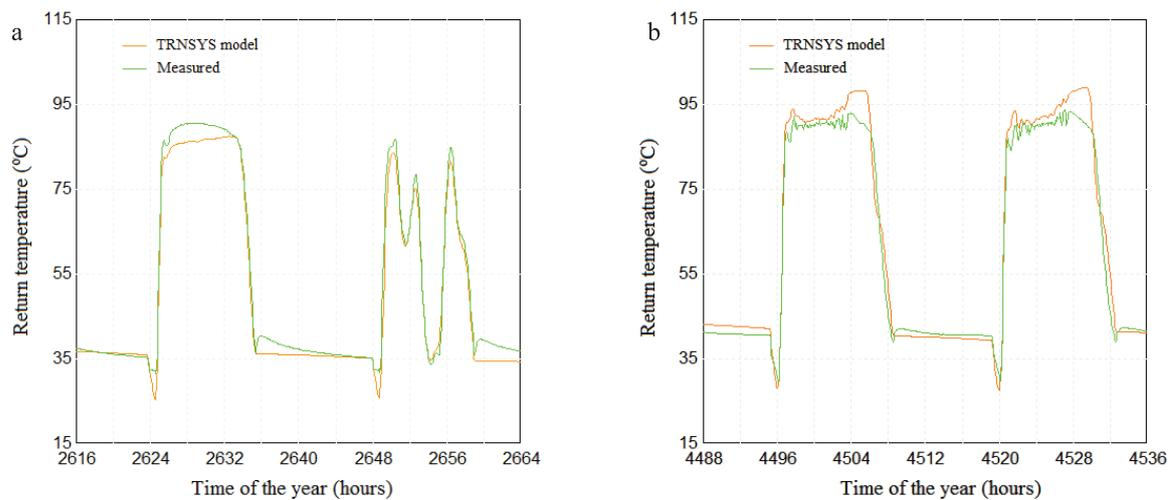
Fig. 4. Comparison between simulated and measured return temperature from the solar collector field: (a) April 20<sup>th</sup> and 21<sup>st</sup>, 2014; (b) July 7<sup>th</sup> and 8<sup>th</sup>, 2013.
