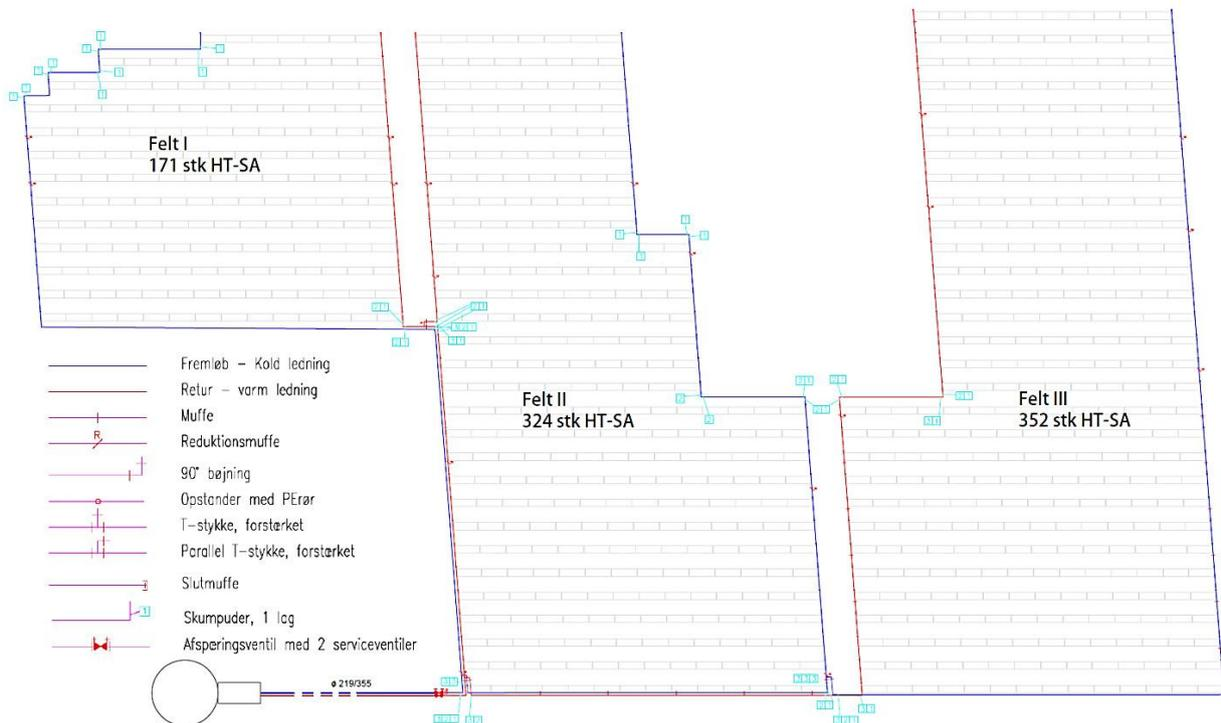
Fig. 1. Layout of the 10,608 m<sup>2</sup> collector field in Braedstrup (source: ARCON Solar A/S).
