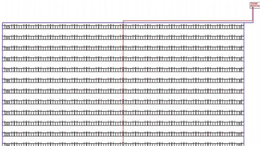
Fig. 2. Layout of Høje Taastrup solar collector field: blue and red lines represent supply and return pipes respectively (adapted from Arcon-Sunmark A/S). (For interpretation of the references to colour in this figure legend, the reader is referred to the web version of this article.)
