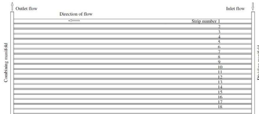
Figure 1.8: Sketch of a typical Arcon-Sunmark collector.
