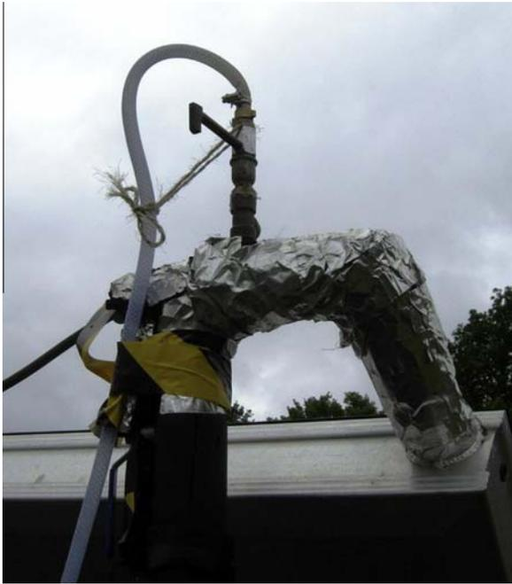
Fig. 3. Detail of collector outlet with connection for the differential pressure sensor.
