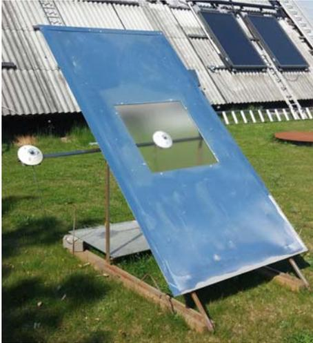
Figure 4.4: Experimental setup for testing the transmittance of a glass pane.
