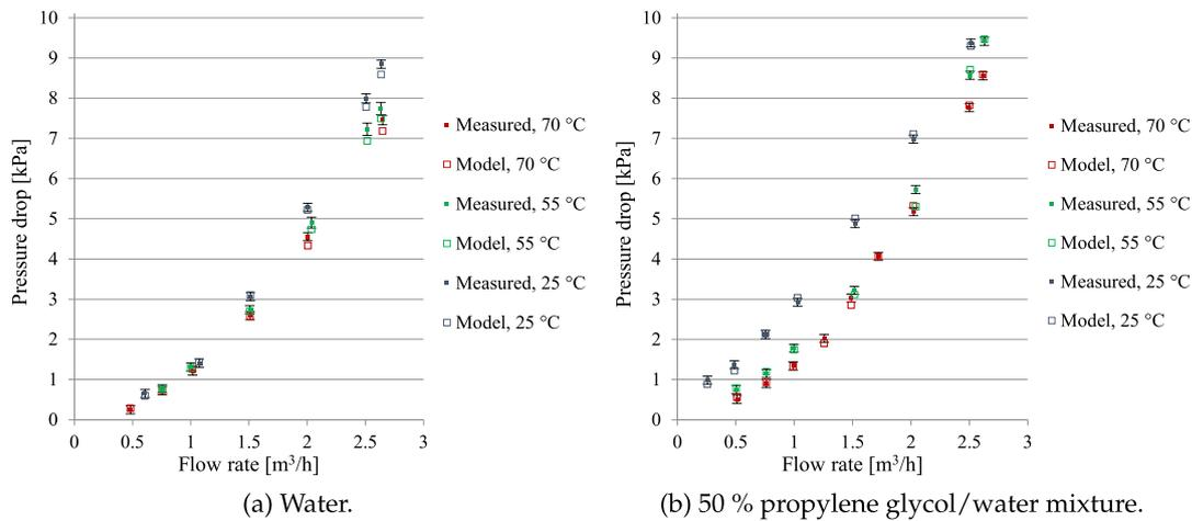
Figure 3.1: Comparison between measured and modeled pressure drops.
