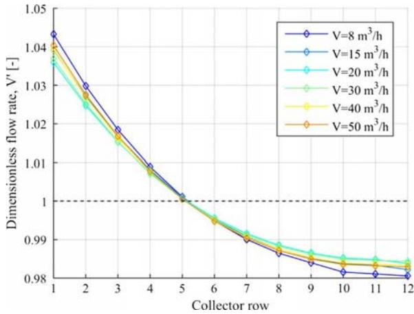
Fig. 13. Modeled flow distributions for different field flow rates in subcase 3.2.
