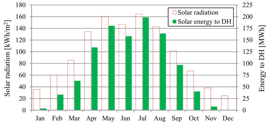
Figure 4.7: Monthly solar radiation on the collector plane (left axis) and energy delivered to the DH network (right axis) in the reference case.
