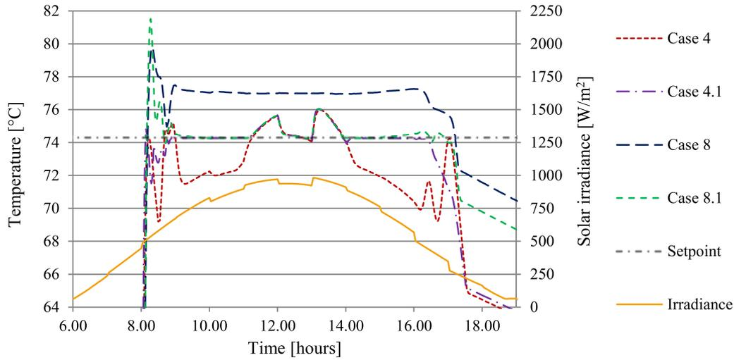
Figure 6: Outlet temperature from the collector field (Cases 4, 4.1, 8 and 8.1) and solar irradiance on the collector plane on June 7<sup>th</sup>.
