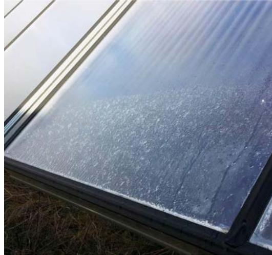
Figure 4.5: Condensation on glass pane of a collector in Høje Taastrup field.
