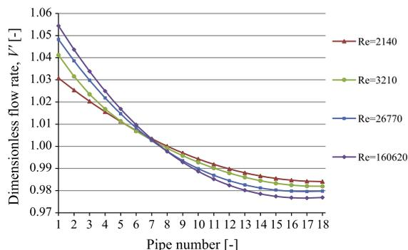
Fig. 9. Flow distribution in the absorber pipes of a HT-SA 35/10 collector for different manifold inlet Reynolds numbers.
