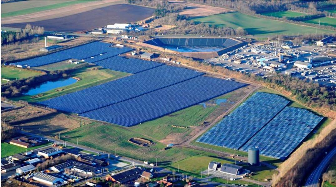
Figure 1.5: Vojens solar collector field with the water pit seasonal storage under construction (source: Arcon-Sunmark A/S).
