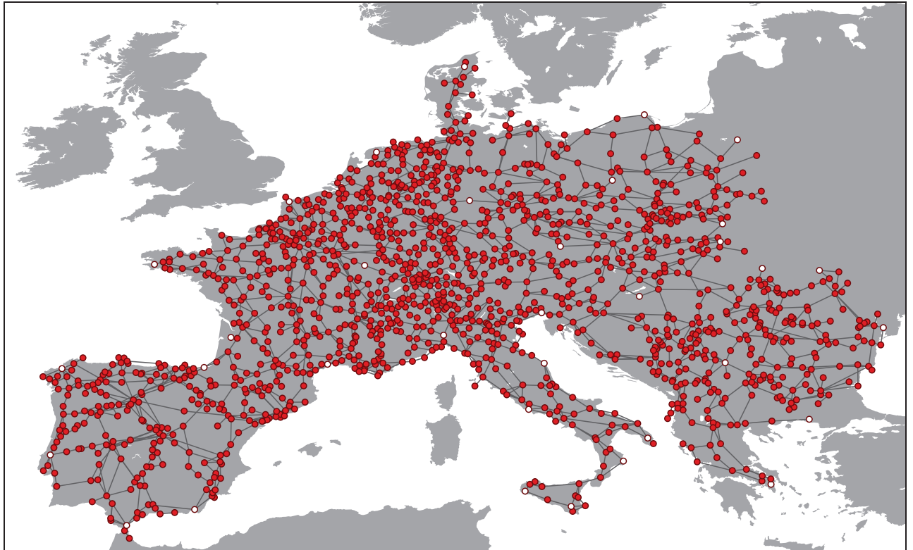
Figure 3. Fitted geographical coordinates for the transmission grid. White nodes are used for fitting the network.
