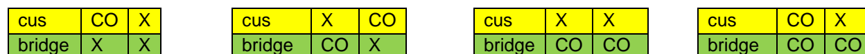
Figure S11: The simulated cell for the \text{RuO}_2 (110) surface with two bridge (site coordinating between two Ru atoms) and two cus sites (on top position on a Ru atom). The four sites are occupied by (a) no spectator: all four active sites can take part in the catalysis, (b) one bridge site blocked by \text{CO}^* , (c) one bridge site and one cus site (closer to the bridge site), and (d) two cus sites and one bridge site filled with \text{CO}^* . Schematic representation of the active site occupation by \text{CO}^* spectators is given below the molecular model, where X denotes an empty site. cus sites are yellow and bridge sites are green. Further, other \text{CO}^* configurations were also studied as follows:
