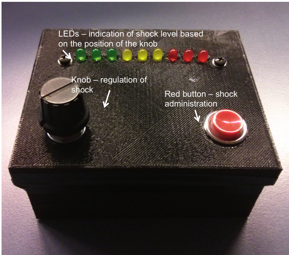
Figure 6.16: Image of the shock generator. The shock generator had a turnable knob that regulated the amount of shock indicated by the coloured LEDs. The red button was used to administer the shock to the robot.
