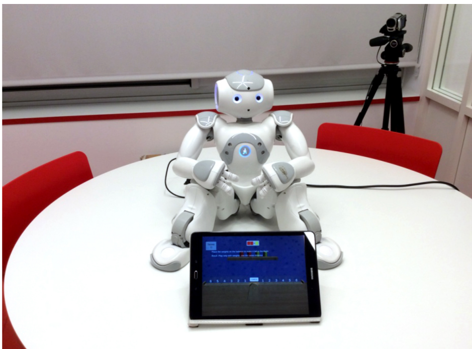
Figure 7.22: The experimental setup. The child sits in front of the robot and interacts with both the robot and the EASELscope. The EASELscope is used to present the different exercises and get the answer from the child. During the interaction, the synthetic tutor (Nao) looks at the child and provides feedback according to the child's actions.
