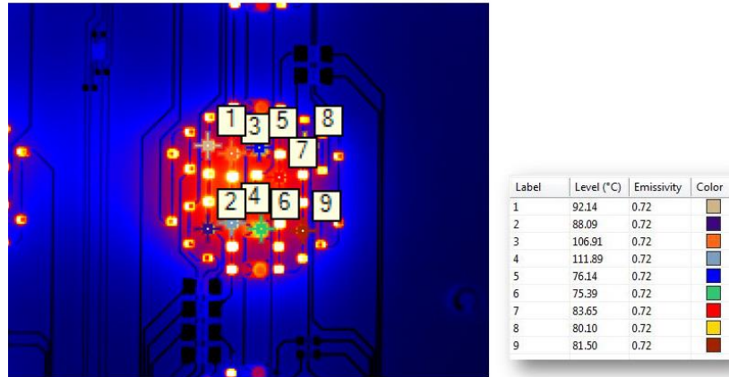
Fig. 4.100. Junction temperatures within one LED cluster of the horticulture luminaire. A maximum temperature of 111.9 °C was measured in channel 5 (PC green).
