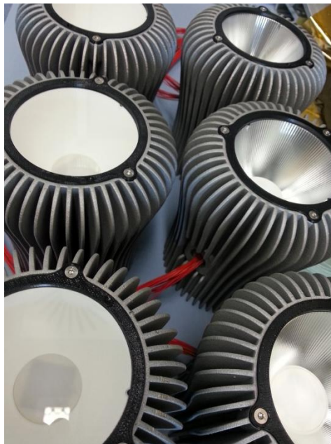
Fig. 4.89. Lamp housings ready to be attached to their matching drivers. Note the difference between the spot and flood reflectors.
