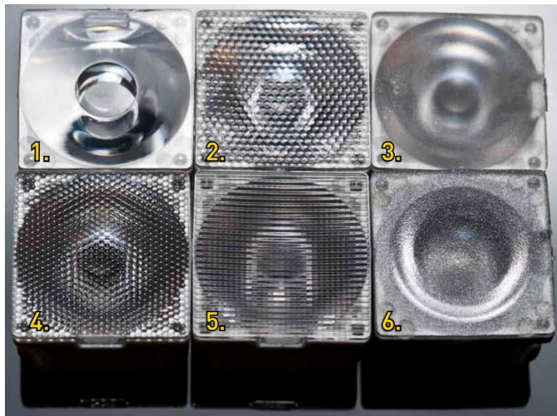
Fig. 4.38. LED optics showing a basic TIR lens with surface patterning to create the final beam profile: Real Spot (1), Smooth Spot (2), Diffused Spot (3), Medium (4), Oval (5) and Wide (6).
