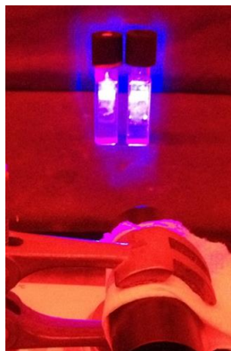
Figure 4.8 Picture of the set-up used for the quantum yield measurements.
