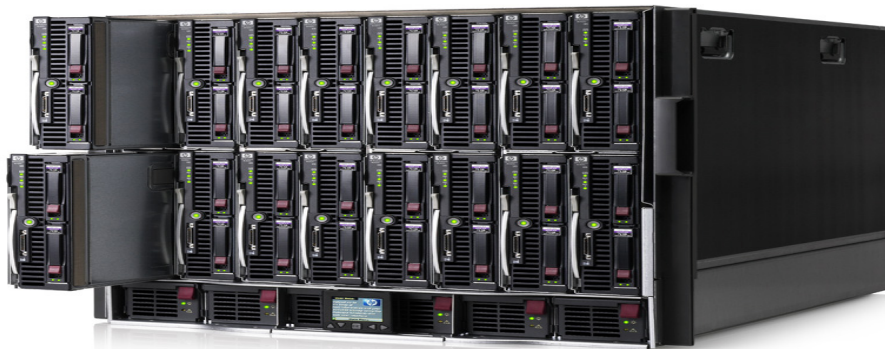
Fig. 2 An HP Blade Enclosure with 16 Blade Servers Installed and a Dedicated PSU at the Bottom [4]
