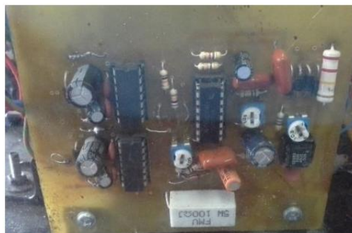
Figure 7: Implementation of Oscillator Circuit Design
