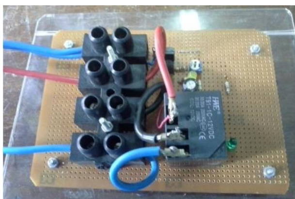
Figure 10: Charge Controller Circuit
